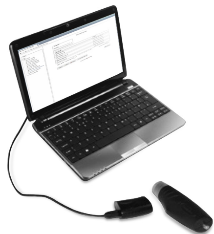
RemoteBook operating on a laptop computer. A Guardus G7 is being downloaded via the USB Download Cable with Infrared.
