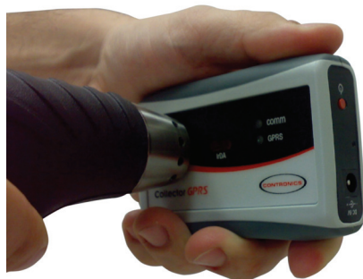
Collector GPRS receiving data from a G3 Guardus to be immediately relayed to the central station by cell phone.
