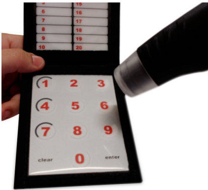
A Guardus G7 reading an RF-Tag Events Wallet.
